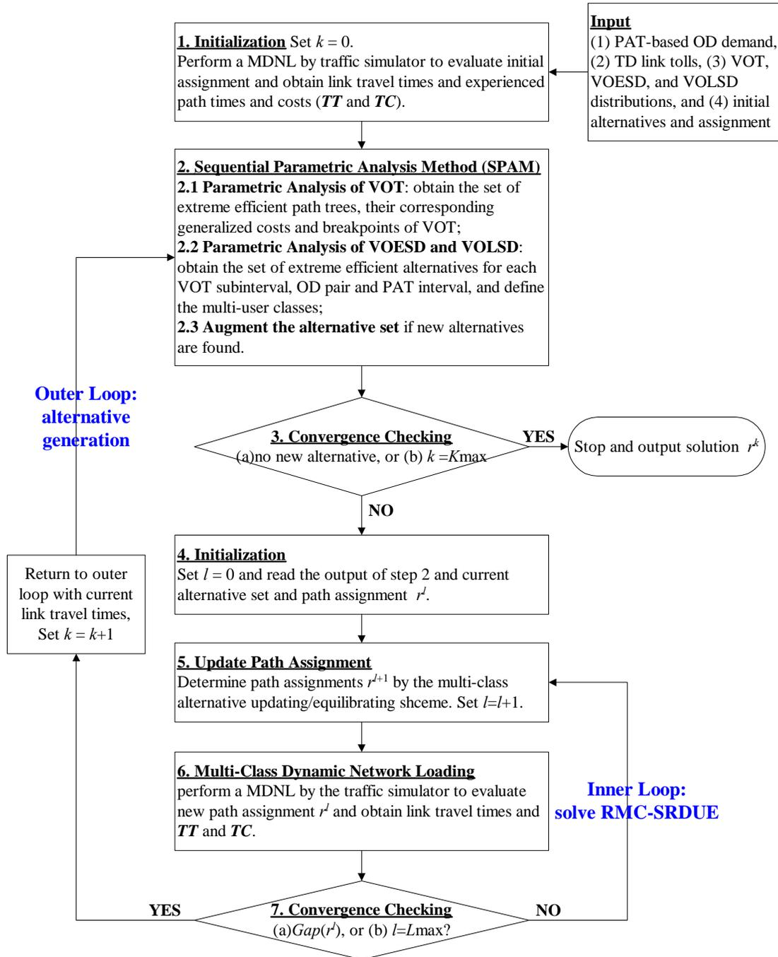
Fig. 1 Flow chart of the MSRDU solution algorithm
