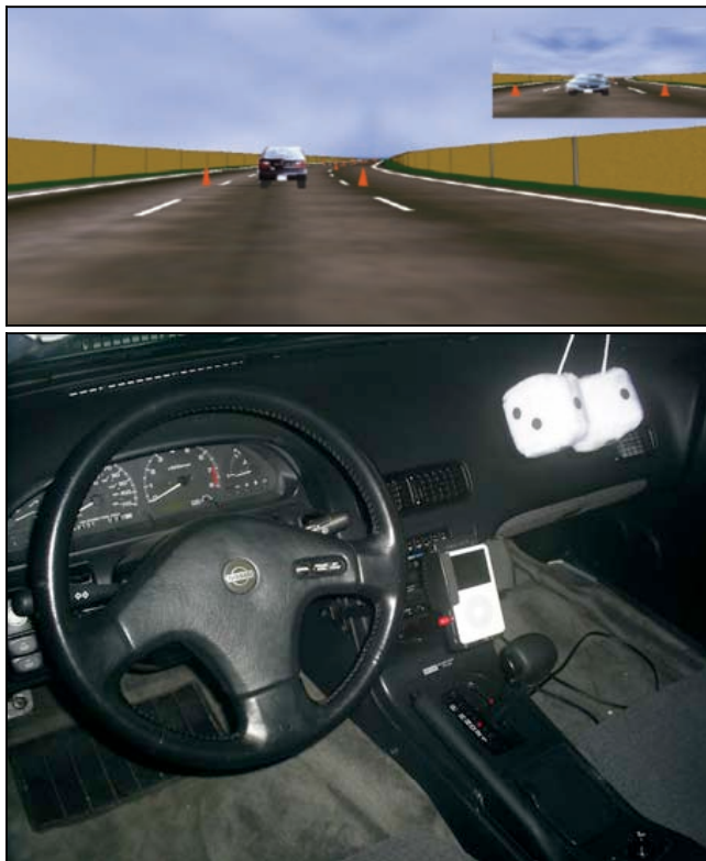
Figure 1. Driving simulator screen shot and interior with in-vehicle iPod mounting.
